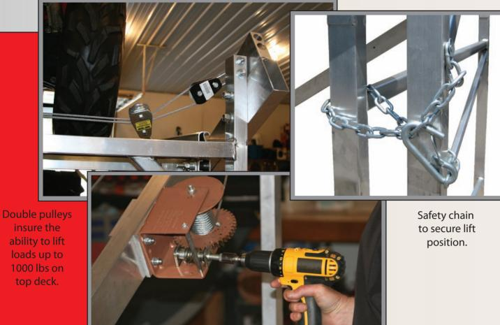
Worm gear winch, attachable on either side of lift for ease of operation.
